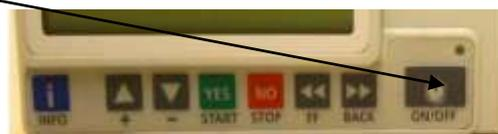
Then press the **ON / OFF** key until the 'Self-Test' screen appears.
